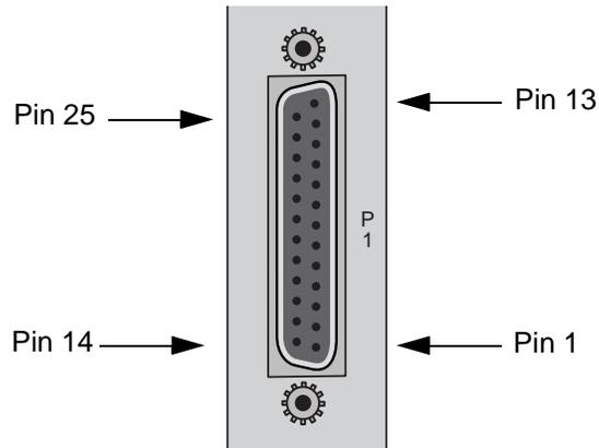
**Figure C-29. HSU-T V35 Card Jack Pin Orientation**
