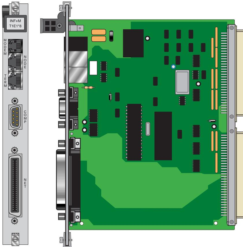
**Figure 6-5. INF+M Interface Card**
