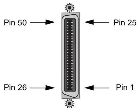
**Figure C-58. P-Phone PPO and PPS Card Tip/Ring Connector**
