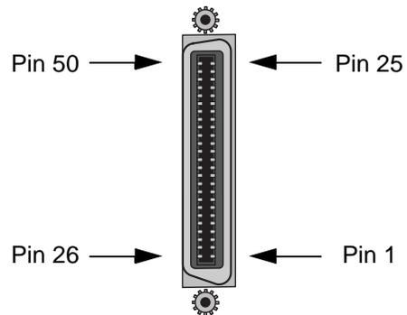
**Figure C-31. Four-Port HSU\*4E 530/35 Card Jacks**
