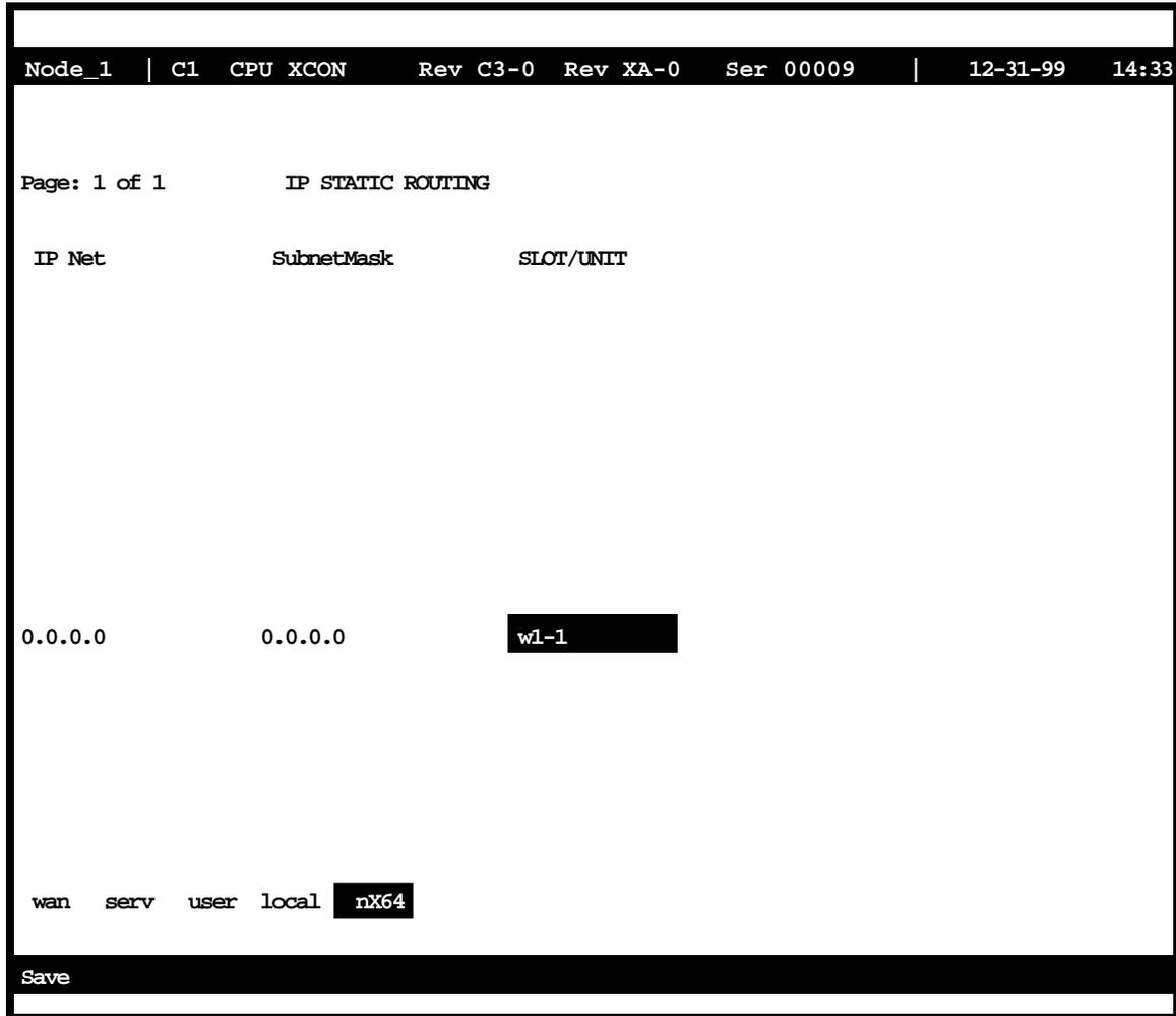
Figure 5-16. Slot/Unit Options Screen
