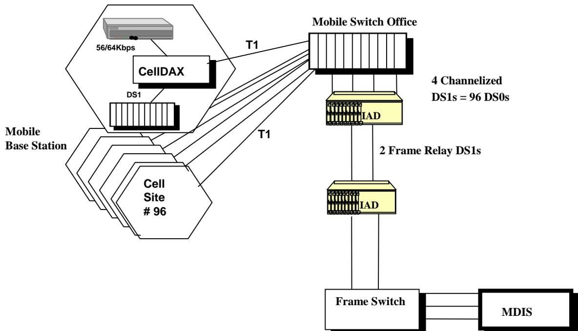
Figure 2-25. Cellular Network Frame Relay Application
