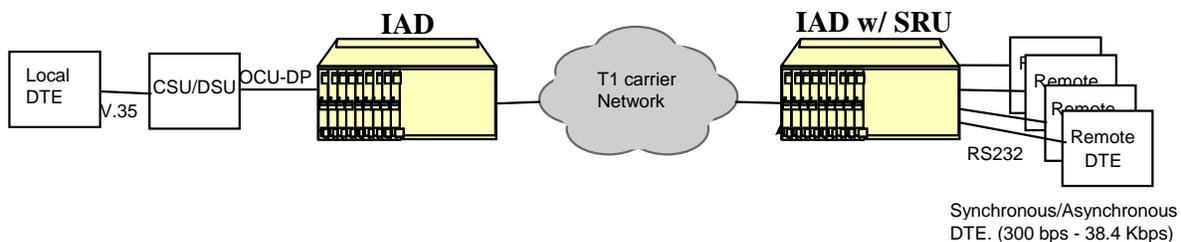
**Figure 2-5. IAD with SRU Card Application**
