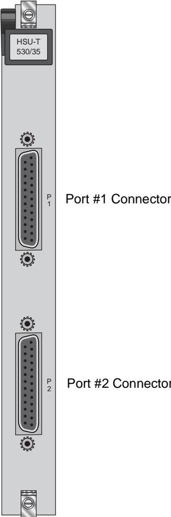
**Figure C-28. HSU-T V35 Card Front Panel Connectors**
