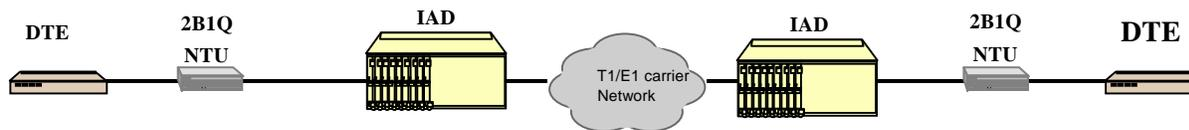
Figure 2-8. BRI Card in a Leased Line or IDSL Application
