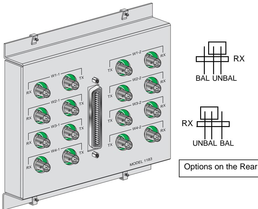
**Figure 7-21. E1 Interface Adapter Panel**
