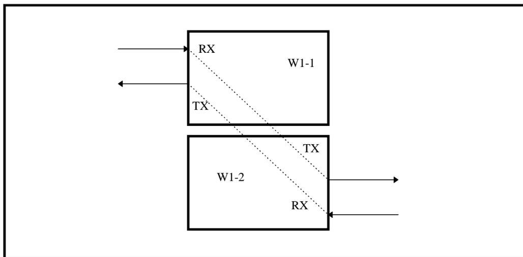
**Figure 7-48. PARS Time slot Cross-connection between Primary and Secondary WANs**
