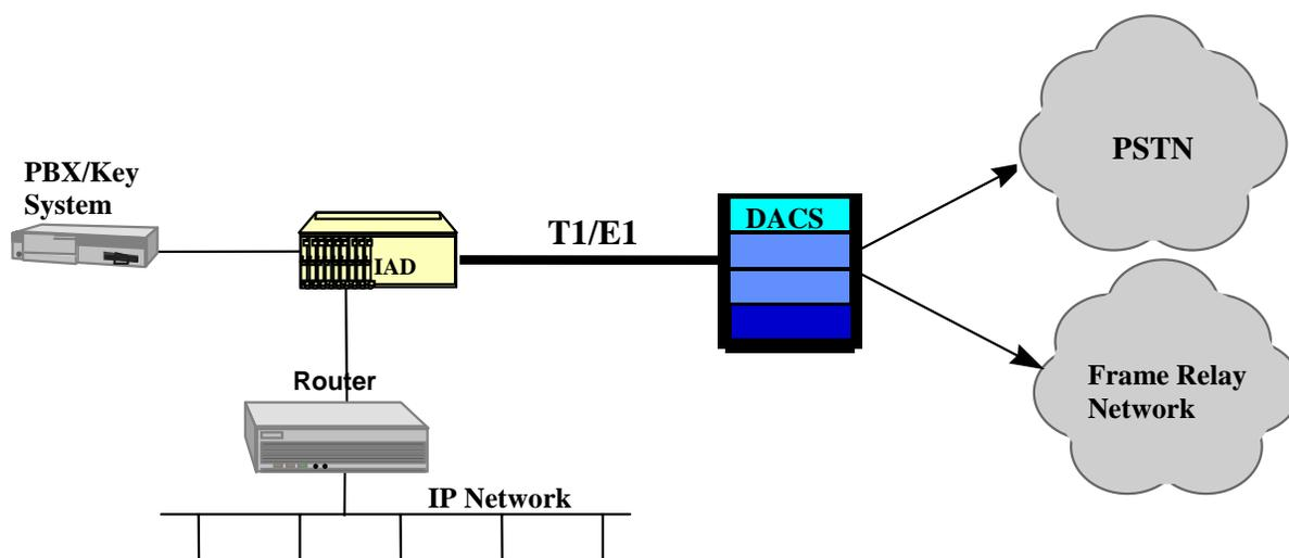
Figure 2-29. IP Routing Server for Internet or Intranet Based Services
