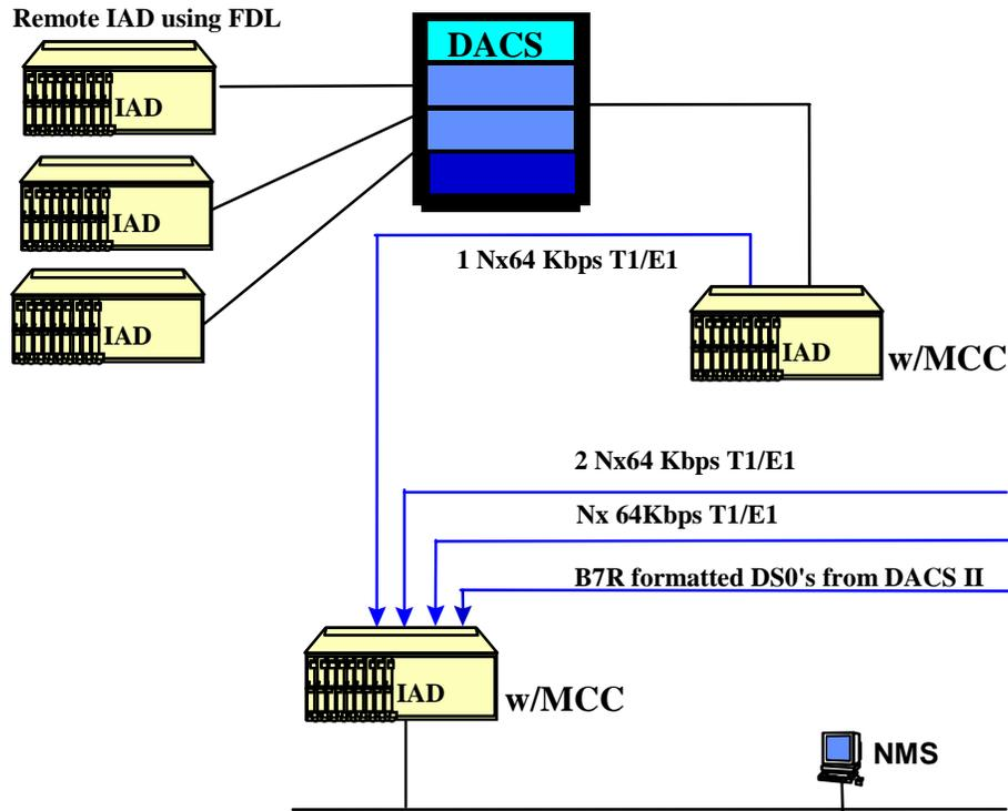
**Figure 2-21. MCC Card in a Multilevel Concentration Application**
