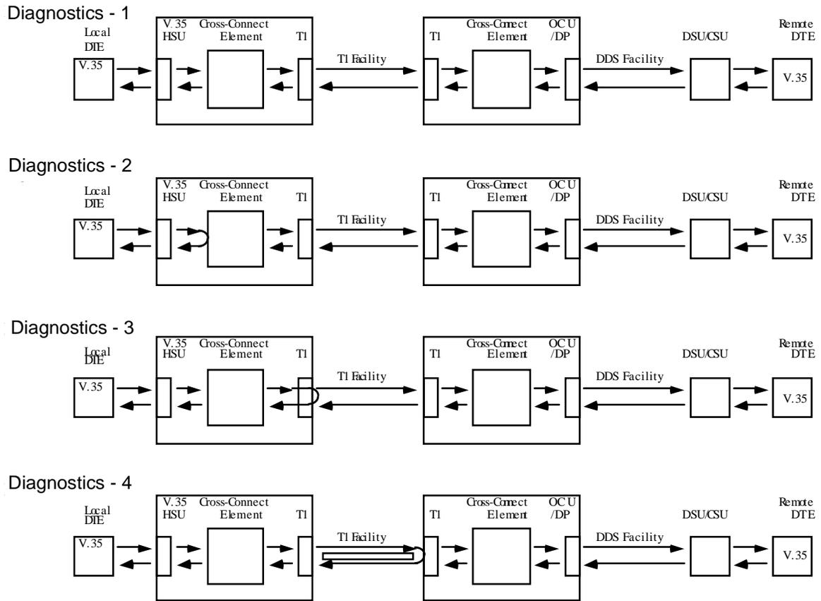
Figure 8-1. Built-In Diagnostics Example
