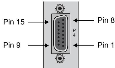
**Figure C-27. HSU-AD 530/35 Card RS-366 Jack Pin Orientation**
