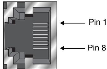
**Figure C-49. IPR 10BT Card Ethernet Port Jack**
