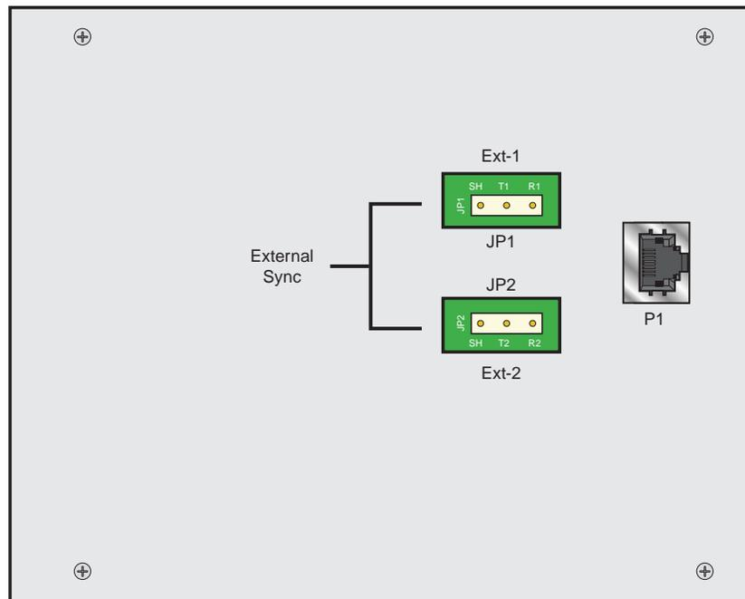
Figure 6-4. External Timing Sync Panel
