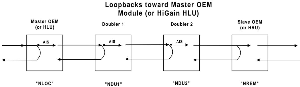
**Figure 7-38. System Loopbacks towards Master Module**
