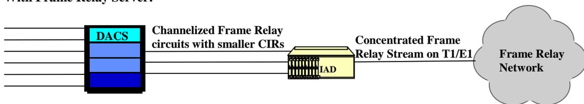
**Figure 2-22. IAD using Frame Relay Server Cards**
