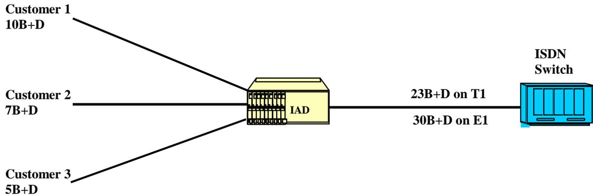
Figure 2-13. Fractional PRI Provisioning using an IAD
