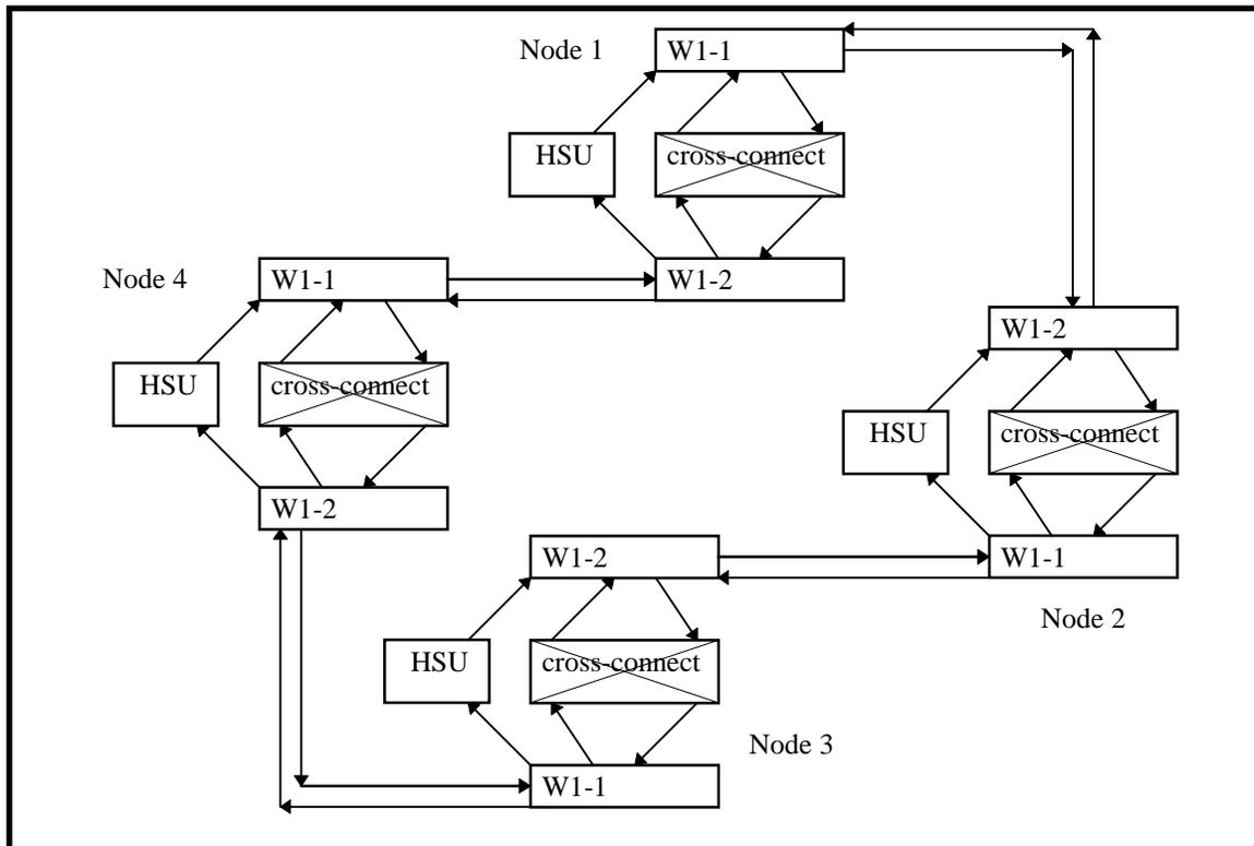
**Figure 7-50. PARS Normal Operation Mode using four IAD Nodes**
