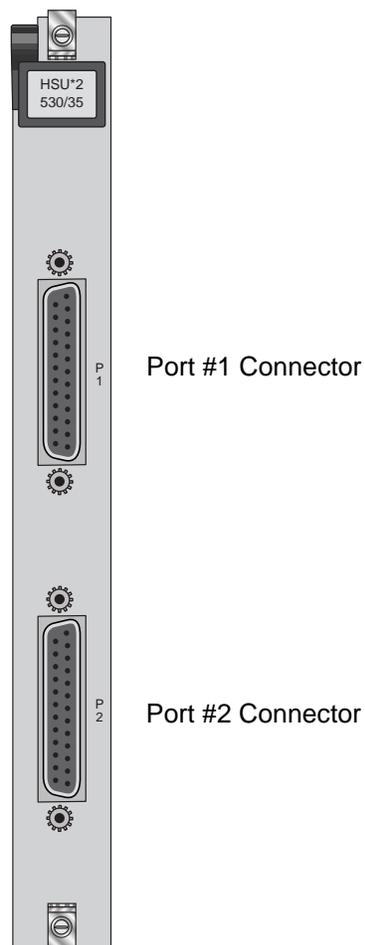
**Figure C-21. Two-Port HSU 530/35 Front Panel Connectors**
