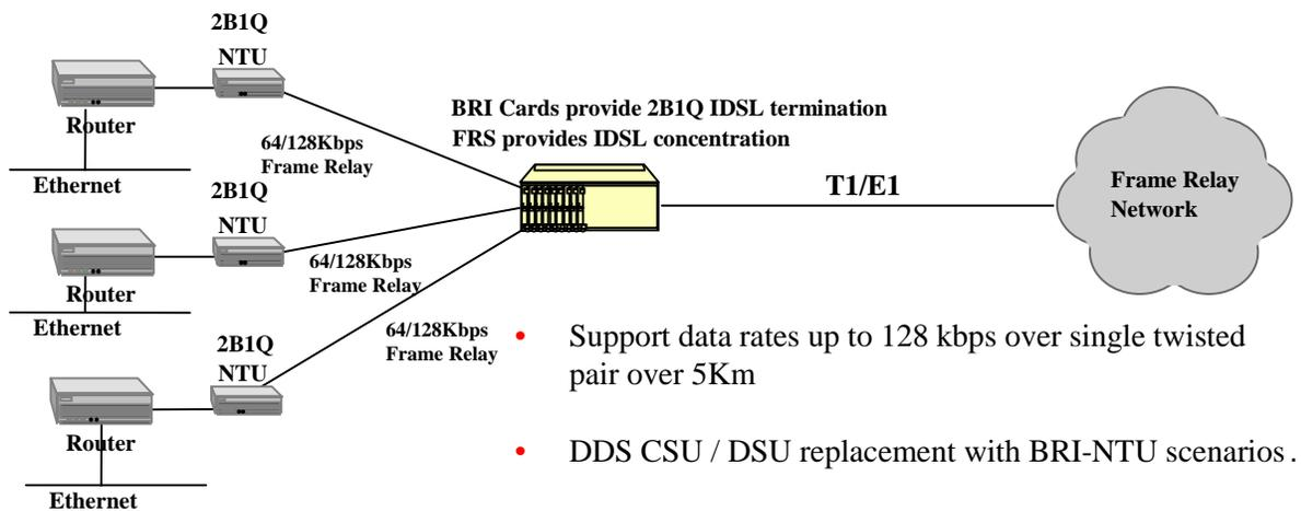
Figure 2-24. IDSL Service Provisioning
