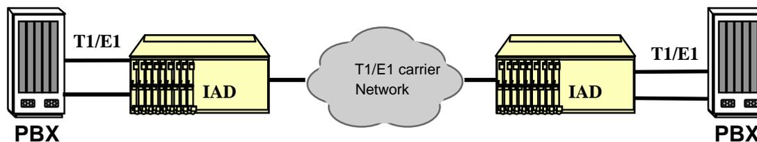
Figure 2-10. IAD using ADPCM for PBX to PBX Application
