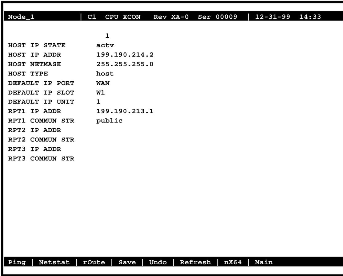
Figure 5-6. Typical TCP/IP Screen
