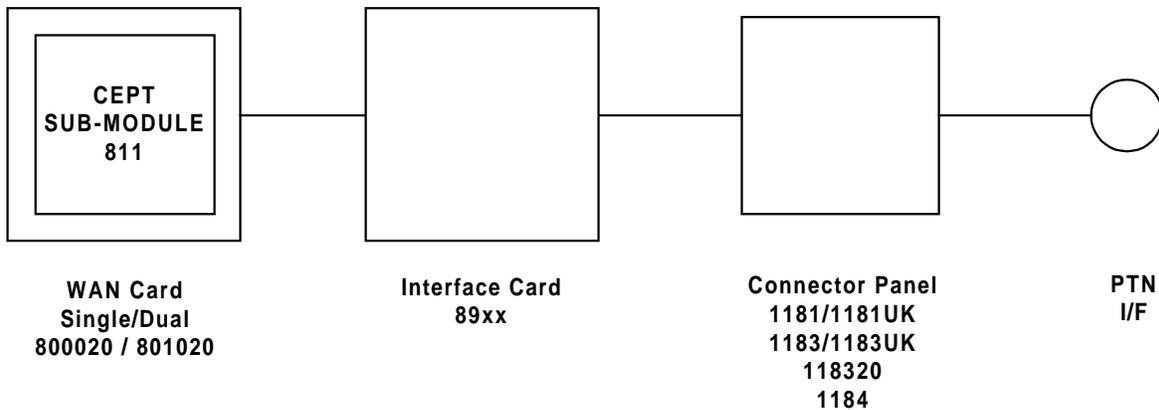
The Interface Card is also listed in the approval documentation and provides a direct metallic path between the CEPT module and appropriate Connector Panel.
