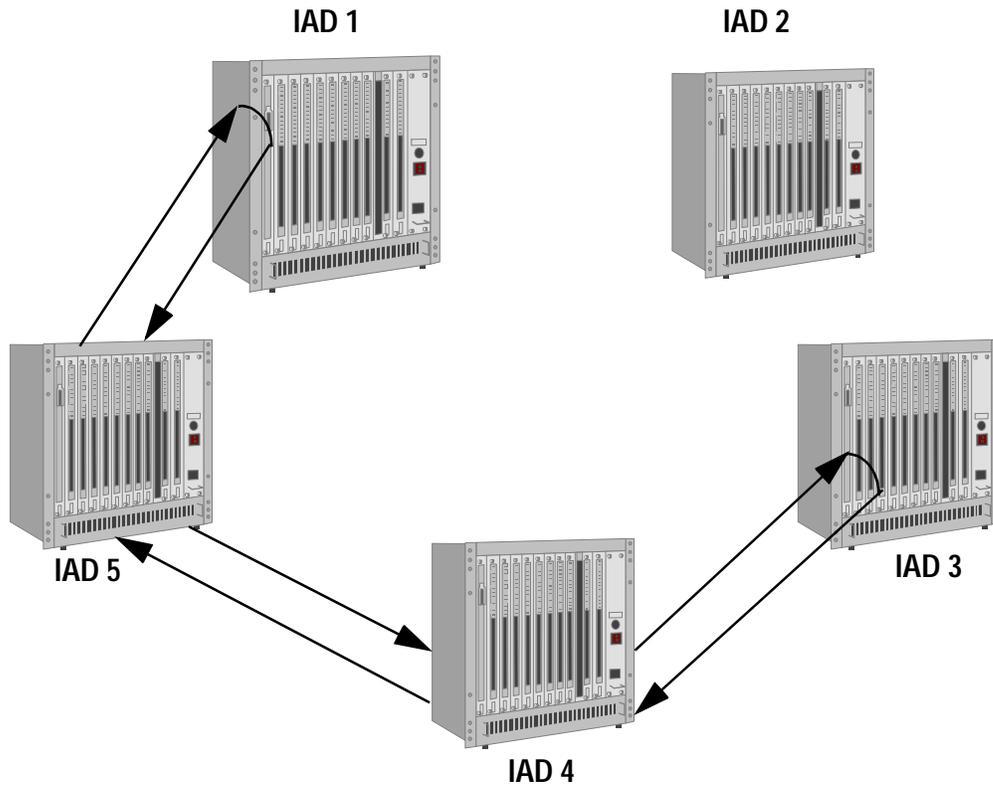
Figure 7-46. Traffic Flow when two Links are Lost (One IAD is Isolated)
