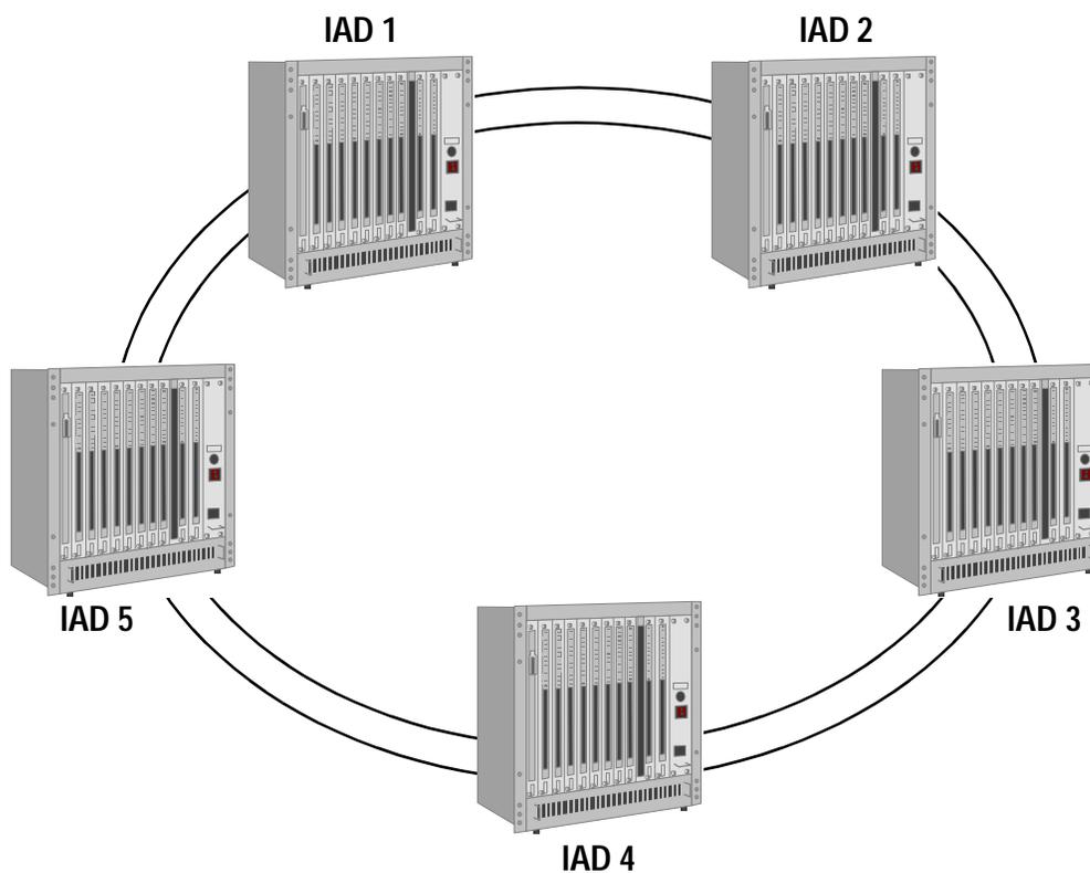
**Figure 7-44. Ring Network Traffic Flow**
