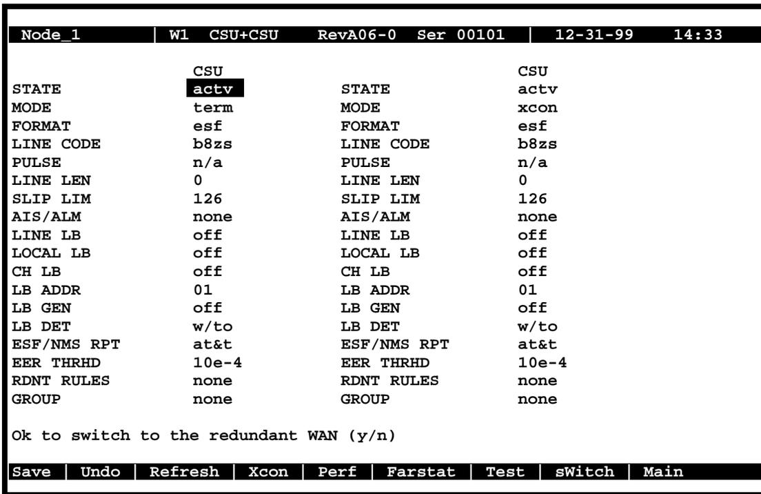
Figure 4-66. Switching to a Redundant Cross-Connect WAN Card
