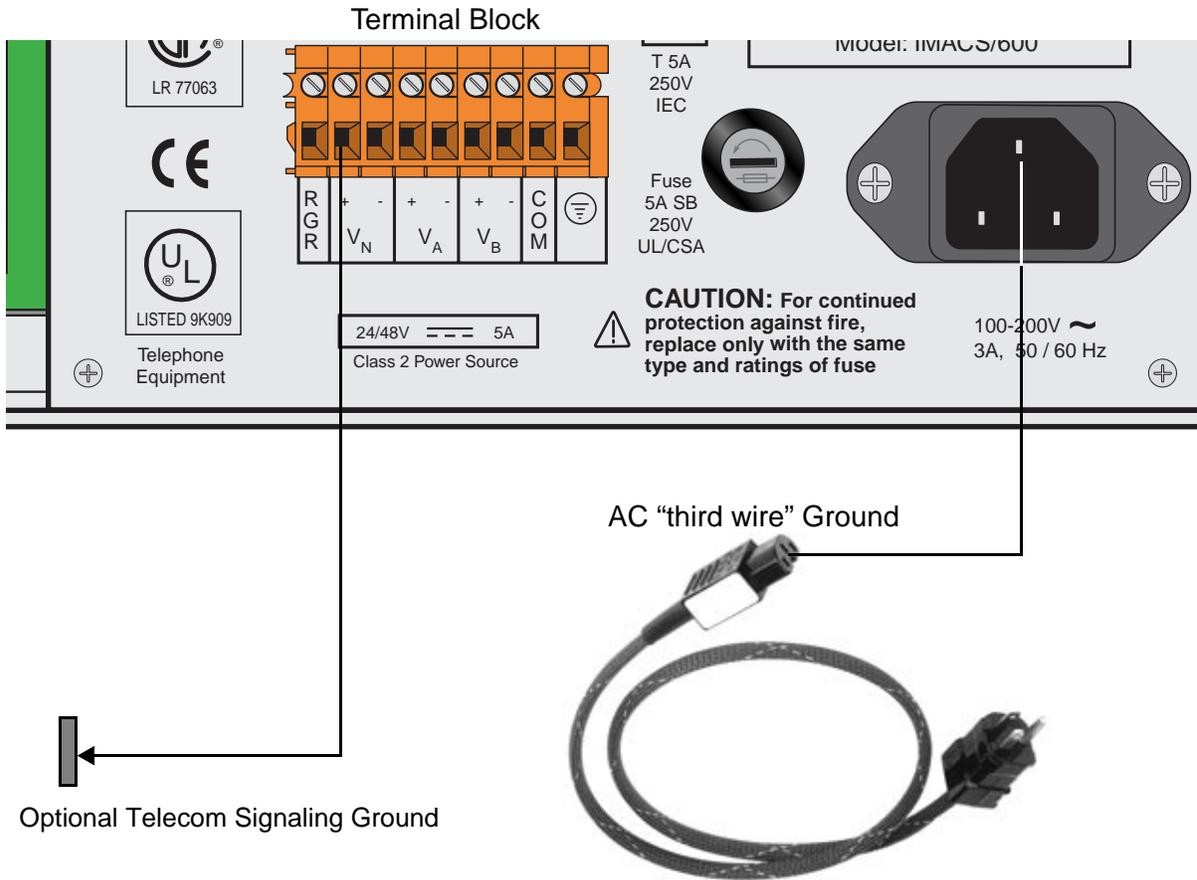
**Figure 3-9. A/C Power Connector on Front-Loading Chassis with Power Supplies on the Side in a A/C Environment**
