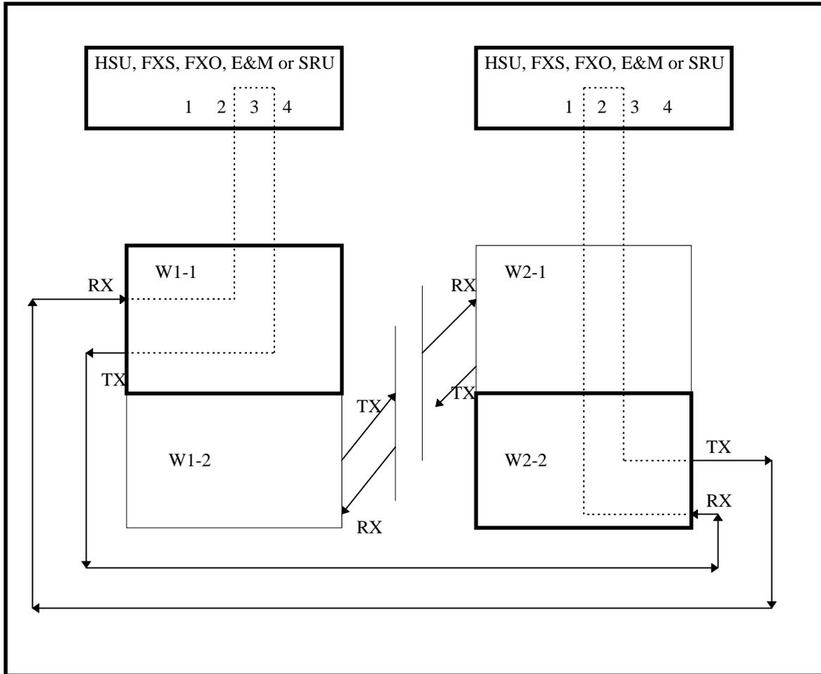
**Figure 7-52. PARS Rerouting (two nodes)**
