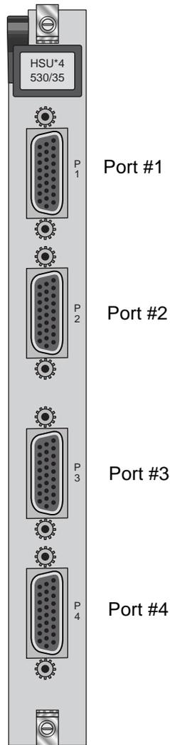
**Figure C-30. Four-Port HSU 530/35 Card Jacks**
