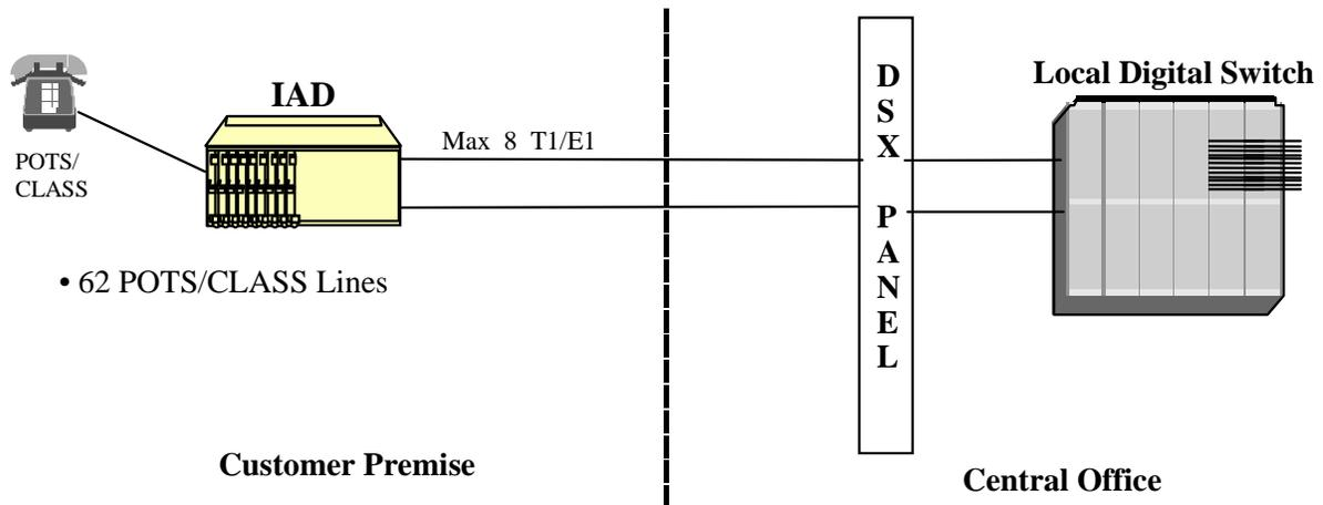
**Figure 2-1. An IAD used as a Voice Channel Bank**
