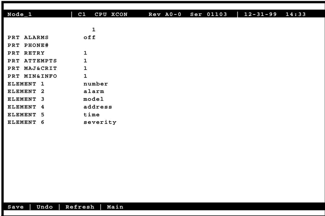
**Figure 5-3. Typical CPU Print Alarm Screen**
