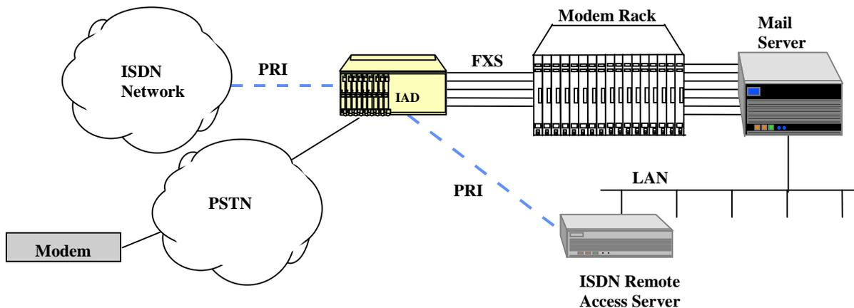
Figure 2-18. PRI to FXS Termination
