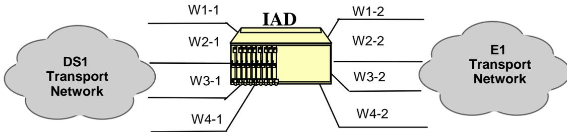
**Figure 2-3. IAD using T1/E1 Conversion**
