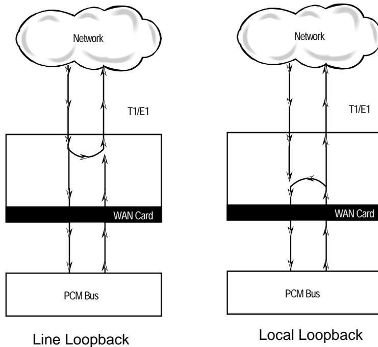
**Figure 7-24. Line and Local Loopbacks**
