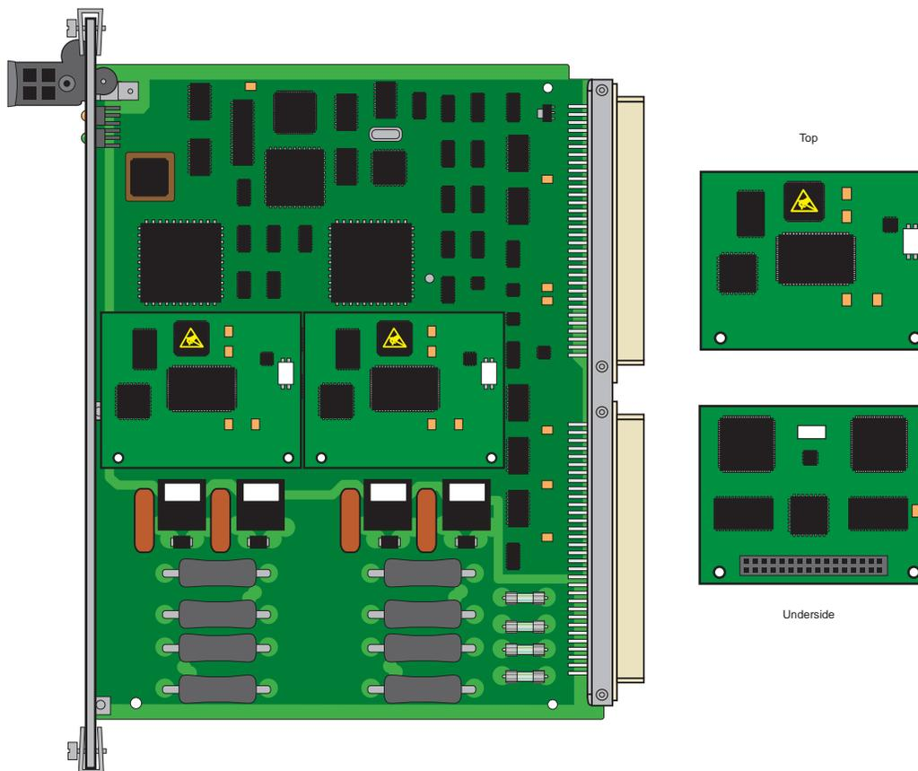
**Figure 7-22. WAN HDSL Card with PairGain T1/HDSL Modules**
