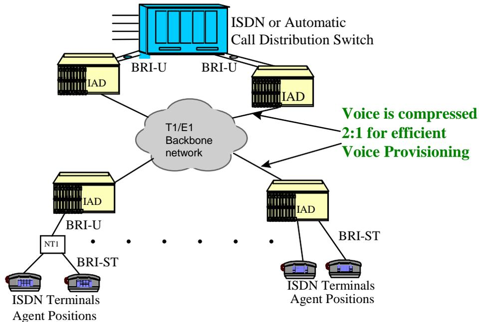
Figure 2-11. IAD in an ISDN-based ACD System
