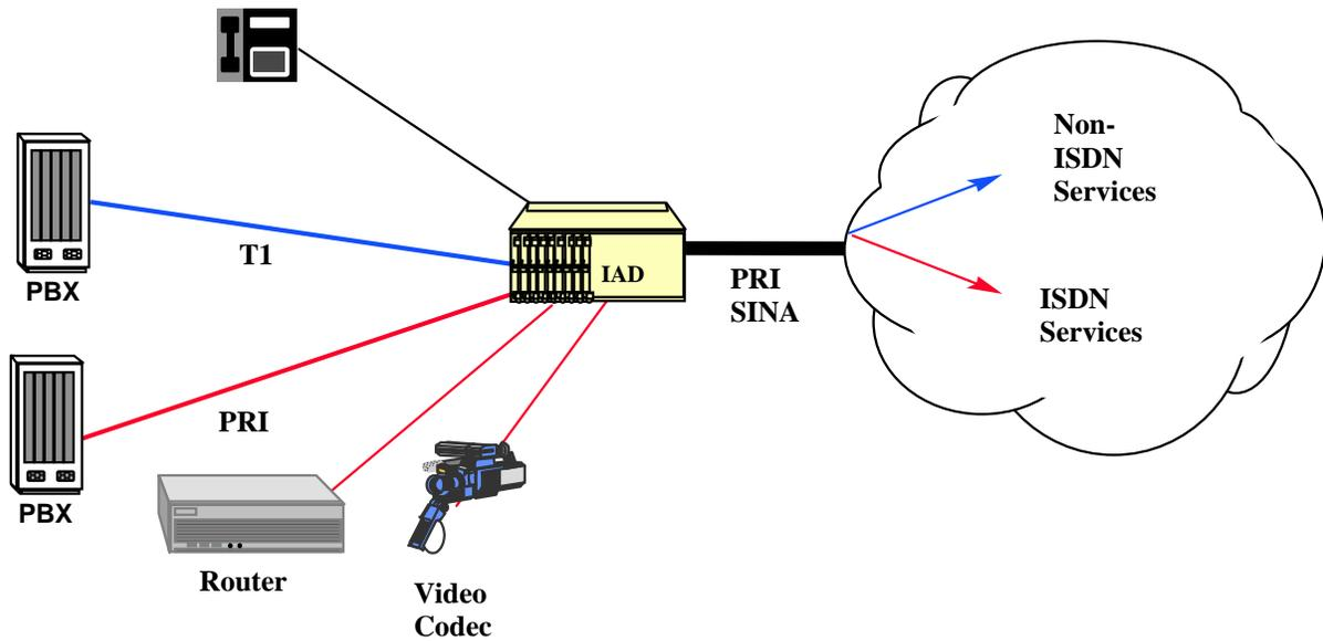
Figure 2-16. IAD using SINA for ISDN and Leased Line Traffic
