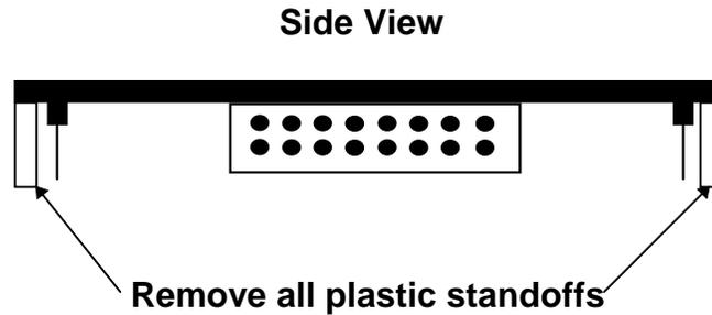
**Figure 7-20. Removal of Plastic Standoffs - 811 WAN Module**
