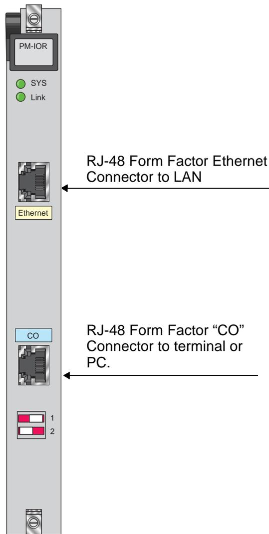
**Figure C-45. RJ-48 Form Factor Card Jacks**
