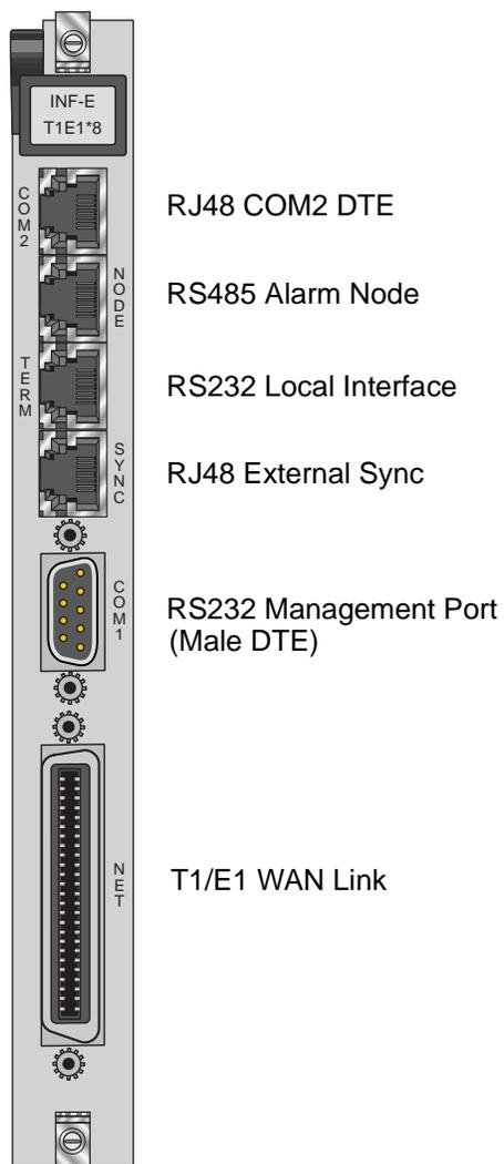
**Figure C-1. INF-E Card Connectors**
