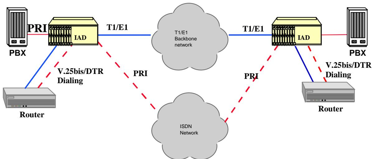
Figure 2-17. IAD using a PRI Server Card for Data Backup
