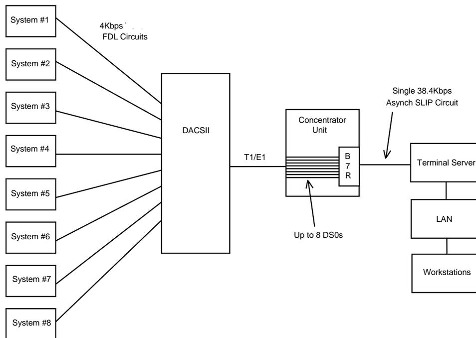
**Figure 5-5. Typical TCP/IP Network Management System**
