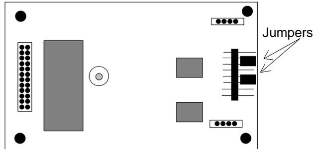
Figure 7-10. DSX/CEPT Revision E+ Module Jumpers
